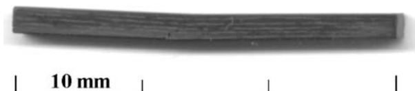
Figure 4 Flexural specimen of basalt fibre reinforced glass matrix composite after rupture; the glass matrix fragments are “bridged” by the reinforcing fibres, without catastrophic failure.
